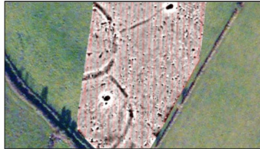
5. GPS tracks (red) highlighting lines of data collection & results from magnetometer fieldwork at a suspected burial ground.
