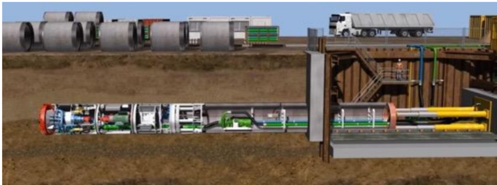
Figure 14 – Typical micro tunnelling set up.
